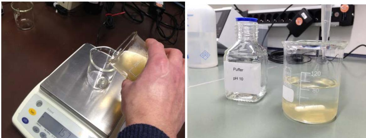
Place the beaker on the magnetic stirrer of the titrator, start stirring and start the method Calcium. The start stirring time is 120 seconds to dilute/homogenize the sample completely in the water/buffer solution:
