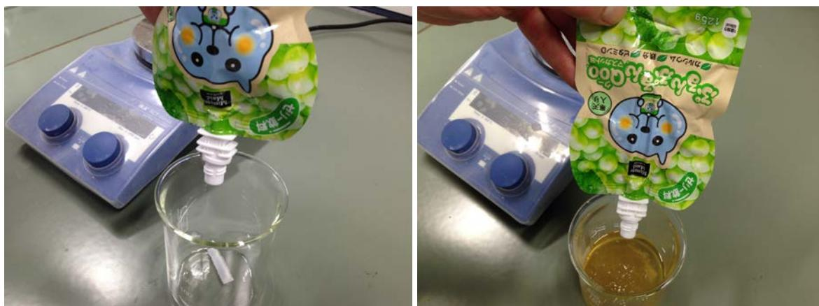
As you can see the sample is complexly homogenous. We stirred the sample at a temperature of 35-40 ° C with a stirring speed of 750-1000 rpm. After 15 minutes the sample is homogenous:
